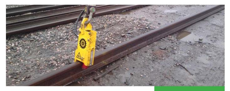
he Thomson Autolok Rail Clamp is available in two versions: the manually operated Autolok M and the hydraulically operated Autolok H.
